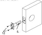
Install latch (5) using wood screws (12) provided.
